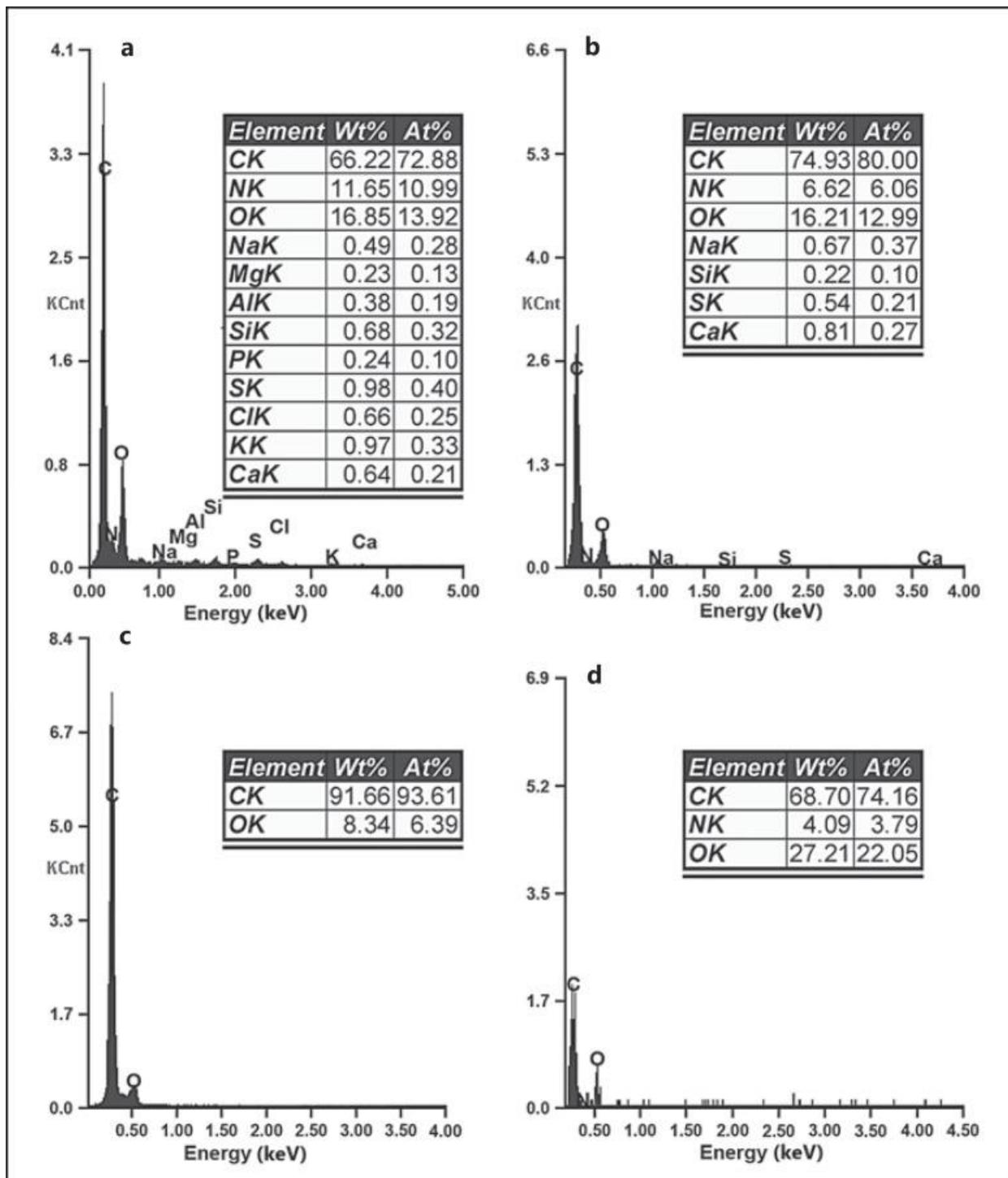
**Fig. 3.** EDX spectra of the nails. **a)** Healthy human nail. **b)** Layer of damaged human nail. **c)** Synthetic nail. **d)** A piece of the damaged nail glued to the synthetic one.
