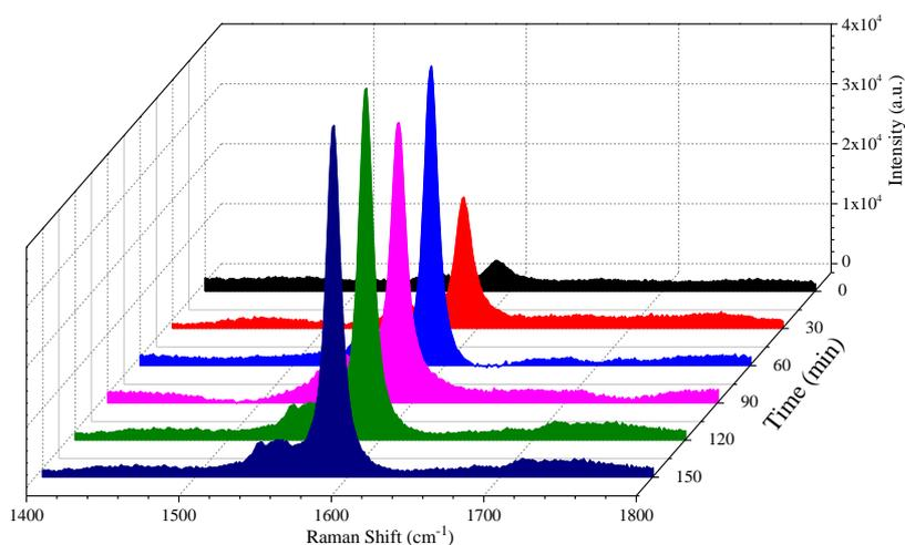
**Fig. 2** Dependence of the Raman signals intensity of SWNT-AuNPs on sonication time.
