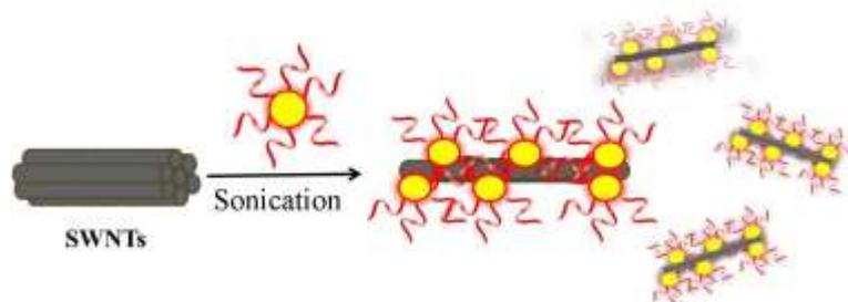
**Fig. 1** Schematic illustration for the fabrication of water-soluble SWNT-AuNPs nanocomposites starting from the DNA-functionalized gold nanoparticles and pristine single-walled carbon nanotubes.
