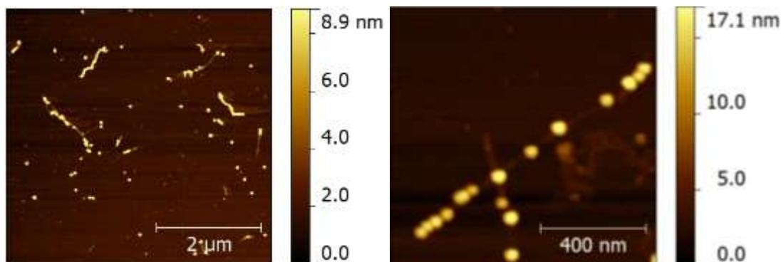
**Fig. 3** Examples of AFM images of the SWNT-AuNPs after 60 min sonication.
